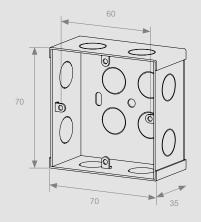
\* Back box type must be defined at the time of order. Unless otherwise specified brackets for UK 3x3 back box will be provided \* Sockets are not comply with EU 2M back box
